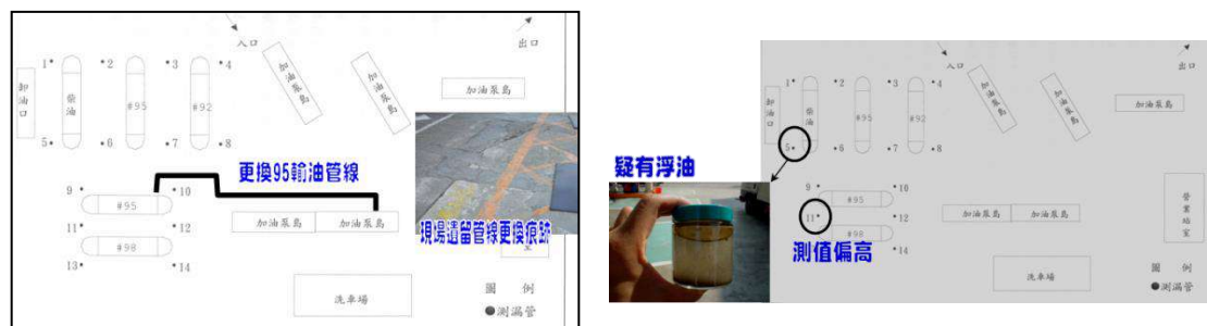
(a) 95 輸油管線更換
